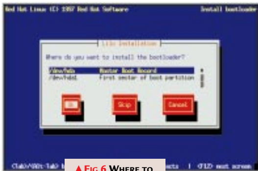
▲ FIG 6 WHERE TO PUT LILO? IF YOU’VE USED DISK DRUID, THE MBR IS PROBABLY YOUR SAFEST BET
